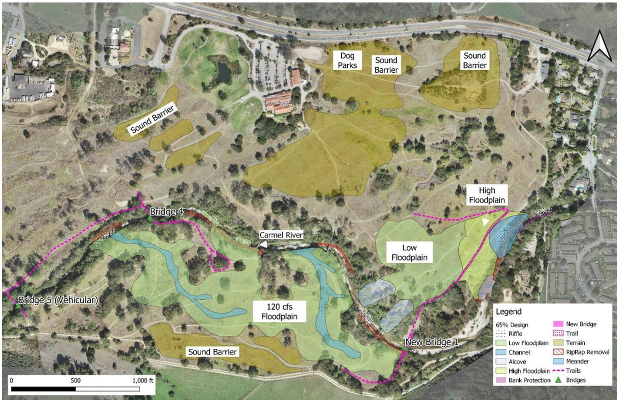
**Figure 2: Project 65% design map illustrating areas of restoration with the floodplain (green and blue zones) and areas where excavated soils will be deposited onsite (brown zones).**
