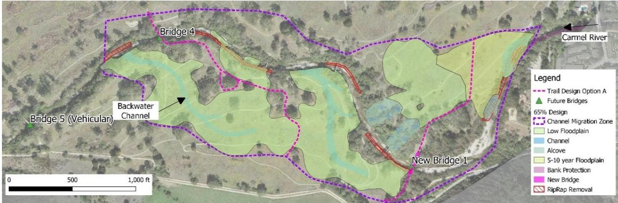
**Figure 4. Trail Design Option A: Trail crossings of the Channel Migration Zone if Bridge 5 is not acquired from adjacent property owner.**
