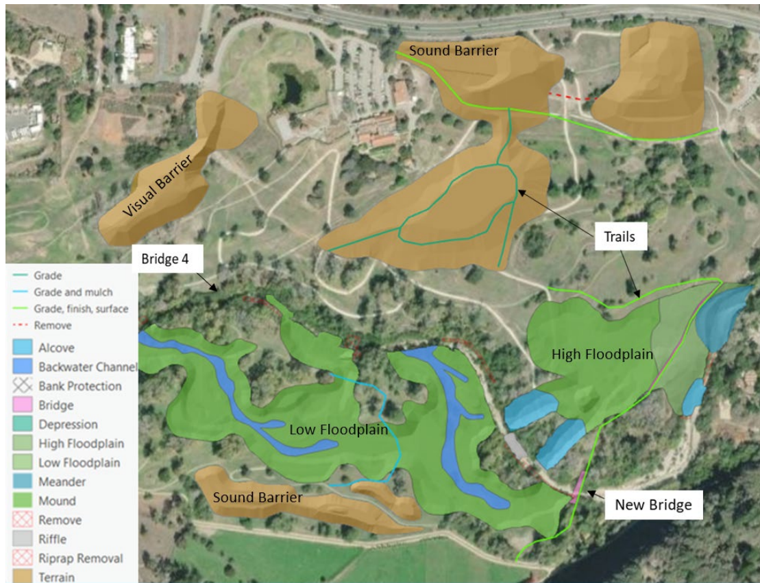
Figure 2: Preferred Project design illustrating areas of restoration with the floodplain (green and blue zones) and areas where excavated soils will be deposited onsite (brown zones) and trail segments that will be constructed.
